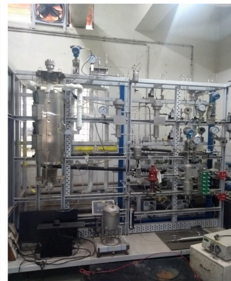
Fixed Bed Reactor
